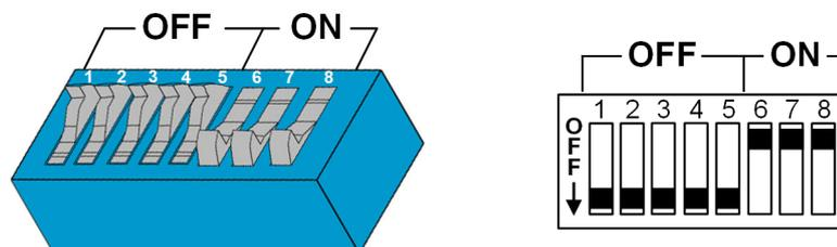
The DIP switches are located under the connection panel cover. The following figure shows only the affected DIP switches, others are not shown. The following setting must be made on the DIP switch DSW2:
