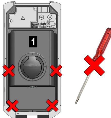
Fig. 1-1: Screws on front part
