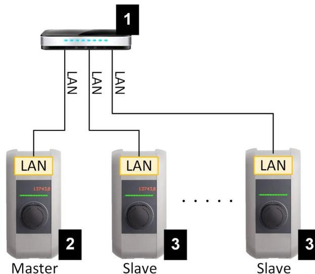
Fig. 2-4: Connection via router or switch
